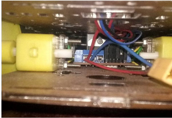
Fig. 3 Bottom layer for motors and motor driver
